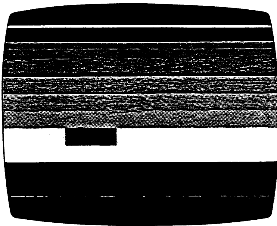
Figure 4-5. Defective Gray Bars Screen
